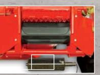
A metal detector in the feed roller is available as an option.
