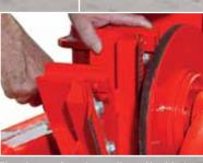
The sharpening stone allows the blades to be sharpened easily and reliably.
