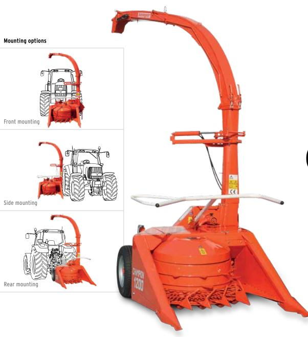
Even on the smallest model, the crop is fed parallel to the chopping blades. This delivers optimum chopping quality. The C 1200 is remarkably compact in construction. Even 90 h. p. tractors can drive the 2-row model. Optimum cutting height is determined by the tractor hydraulics. The stabiliser wheel at the side protects the harvester from contact with the ground.
