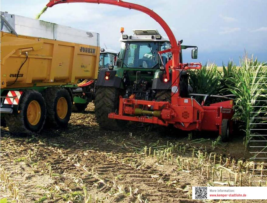
Whether mounted at the front or the rear, the C 2200 3-row model can chop maize. The gauge wheels at the side protect the harvester from contact with the ground. Separate, hydraulic cylinder provides optimal adjustment to the cutting height. The C 2200 consists of the header and the chopping unit with a spout as one compact unit. A maize harvesting header or a grass pick-up can optionally be mounted. A metal detector is available as an option.
